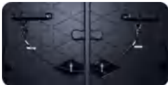
Module safety lock design--Prevent modules from dropping during maintenance
