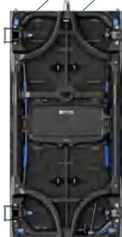
Safety rope design in power box--Better wind resistance
